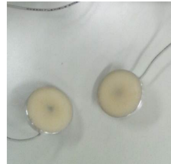
Fig. 5 Adhesive NAM microphone.
